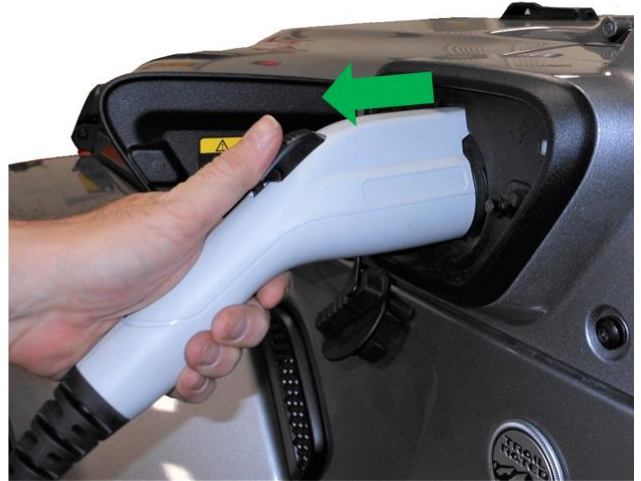
Remove EVSE AC power from the vehicle.
