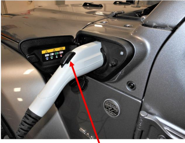
Press the EVSE Recharge Coupler button and pull to remove.
