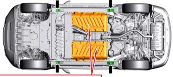
Danger: High Voltage Batteries Do Not Lift or Apply Force Here
