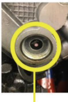
Overheated Pink Sensor 255°F Coolant Temp
