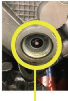
Overheated Pink Sensor 255°F Coolant Temp
