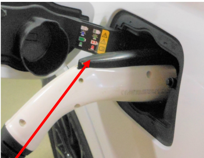
Press the EVSE Recharge Coupler lever and pull to remove.
