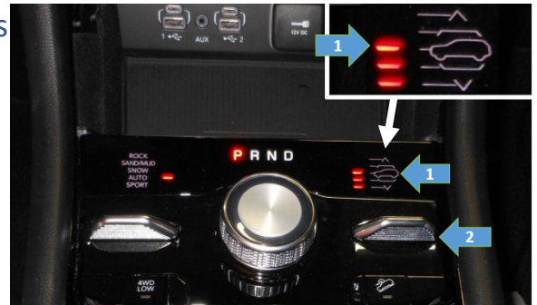
1- Normal Ride Height 2- Ride Height Toggle Switch
